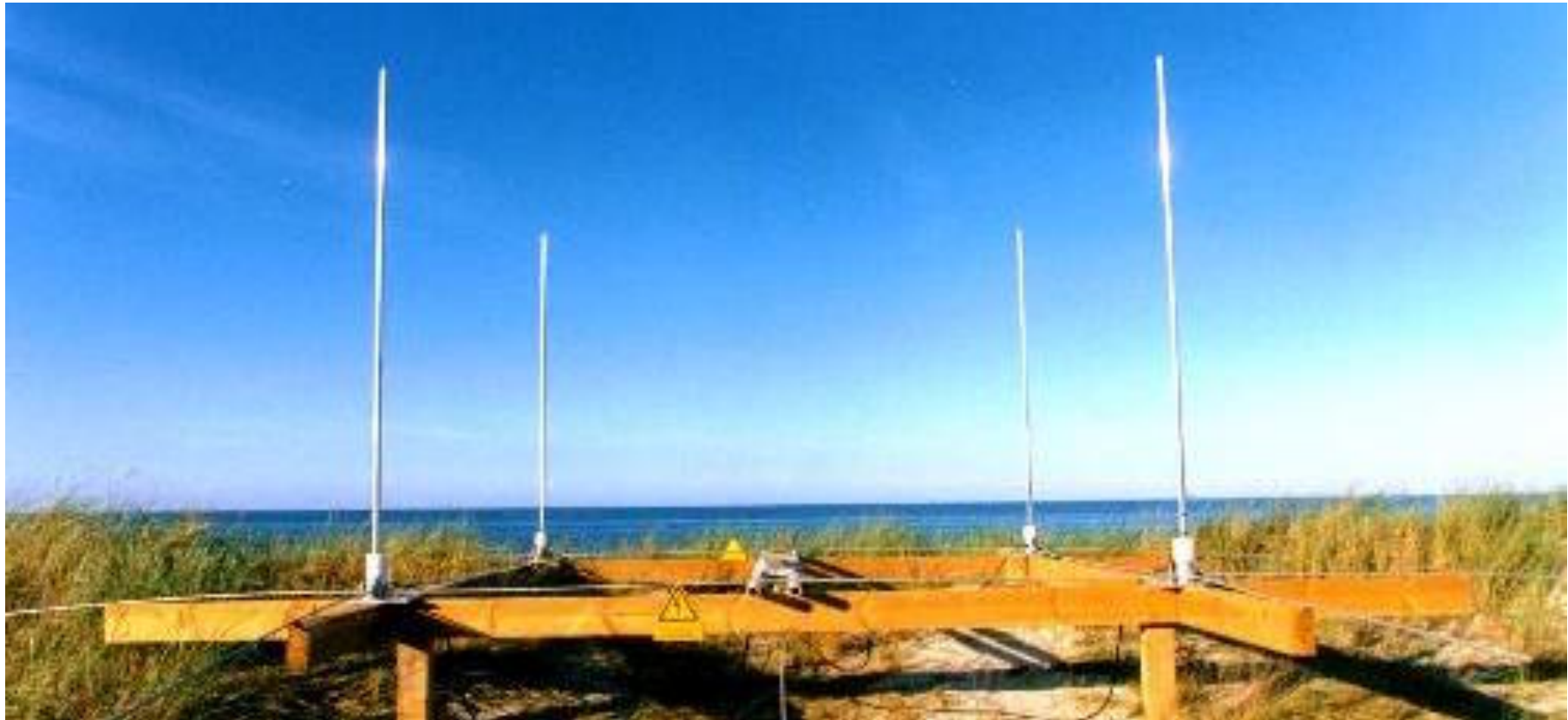
4-element square array receiver
